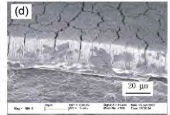
Nanowire coated surfaces Chen et al. Nano Lett., 2009
